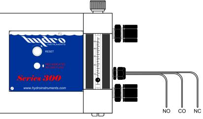
initial status of the alarm switch to be normally open, and connecting NC and CO will set the initial statues to be normally closed. The reversal of the alarm switch state indicates that the chemical supply source is empty.
